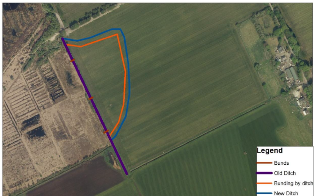
Figure 1. Preferred Drainage Route
