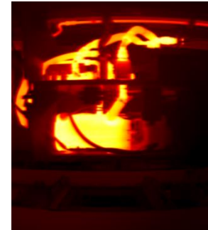
Thermal image of the train underside, showing the operating temperature of difficult to access components.
