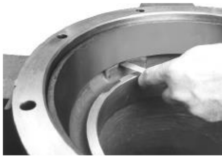
Figure 21: Drive End Outer Race Seating Check
