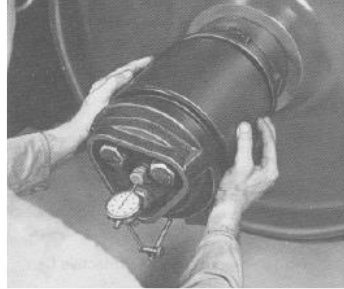
Figure 31: Checking axle bearing end float
