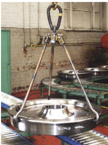
Figure 4: Lifting wheel pan with 3-point lift
