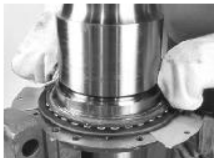
Figure 26: Non-Drive End Inner Spacer Ring Assembly
