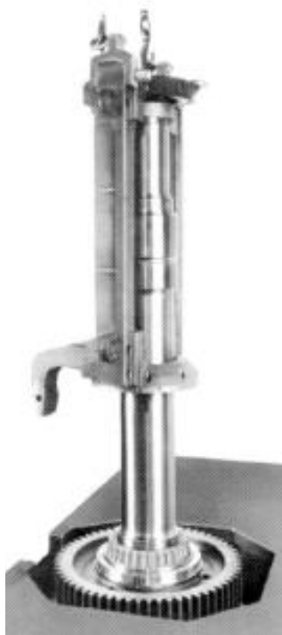
Figure 23: Assembly of Suspension tube to Axle
