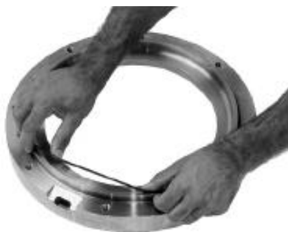
Figure 19: Drive End Bearing End Cover
