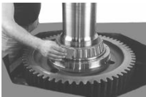
Figure 20: Drive End Inner Race and Roller Assembly
