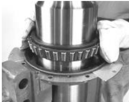
Figure 25: Non-Drive End Inner Race and Roller Assembly
