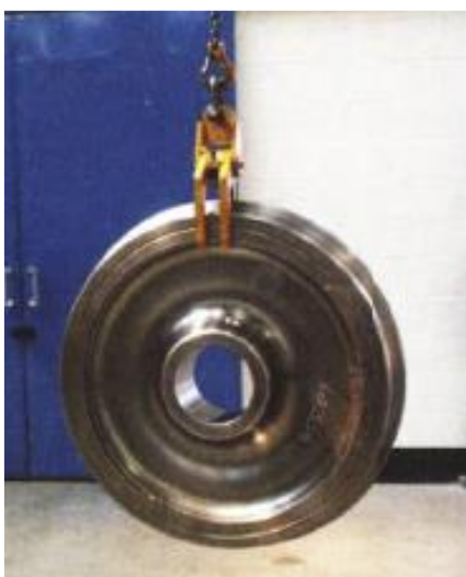
Figure 3: Lifting wheel pan with scissor clamp
