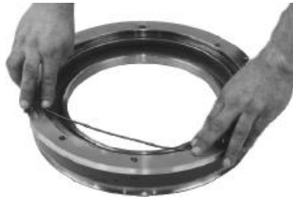
Figure 27: Non-Drive End Inner Bearing End Cover
