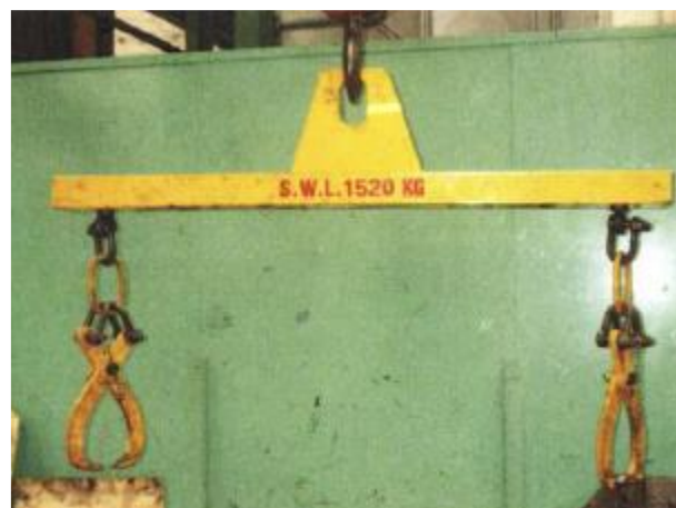
Figure 2: Lifting beam with scissor clamps secured by locking pin
