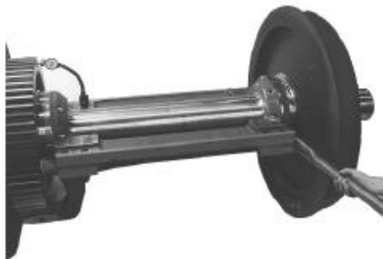
Figure 10: Suspension Tube Bearing End Float Check (different suspension tube is shown)
