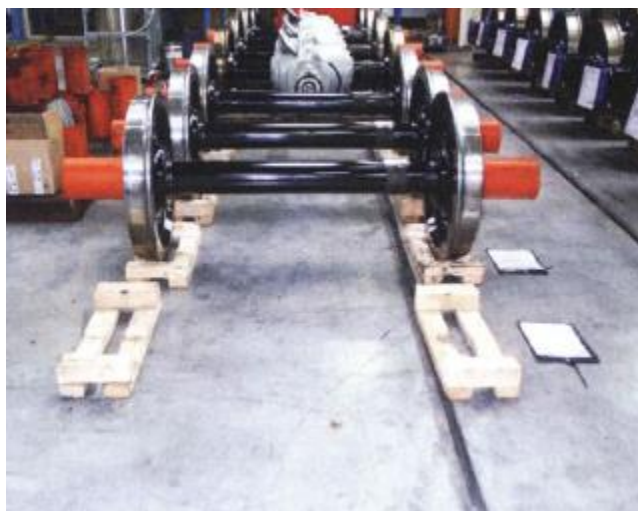
Figure 5: Wheelset storage on concrete
