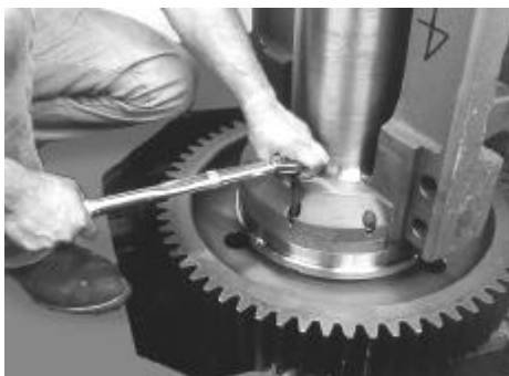
Figure 24: Bolting of DE bearing end cover to suspension tube
