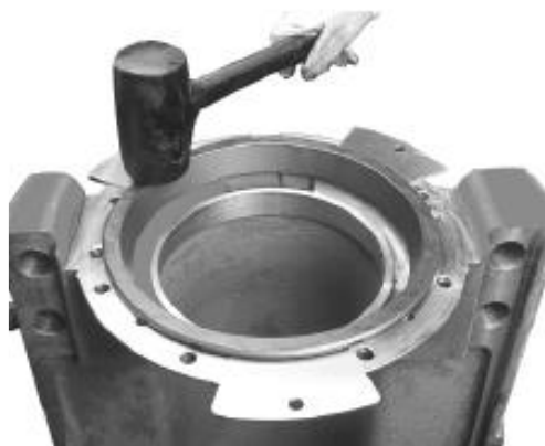
Figure 22: Seating of Non-Drive End Outer Race
