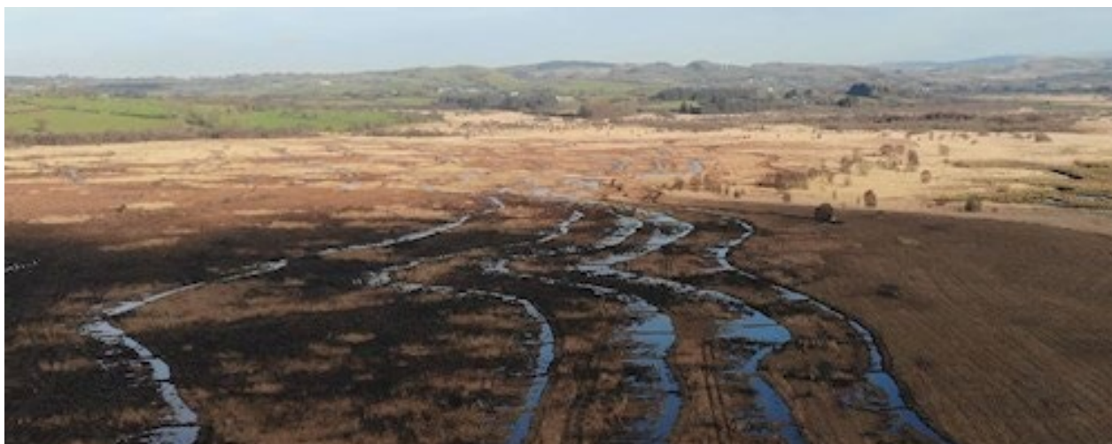
Figure 4 Cors Caron low contour bunds. Photo credit: Natural Resources Wales
