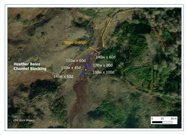
The intention of the blocks is to cause backing up of flow which then spills outside of the channel onto the adjacent valley floor, creating shallow flow over the surface. In addition to spilling flow, the bales prevent a downstream transport of sediment and leading to a natural infill of the channel to raise bed levels.
