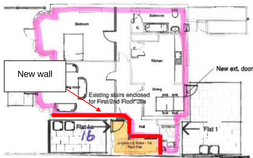
Figure 1 - New separating wall
