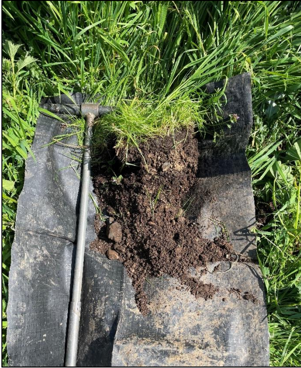
Figure 38. TP1 – Sandy loam topsoil mixed with stones and made ground.
