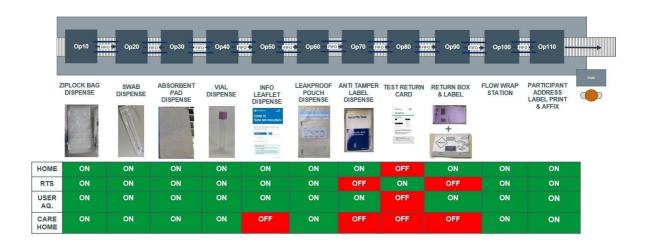
Fig.5 - Primary Kitting Cell Initial Concept.
