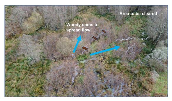
At the point where the current straight channel is most central to the drainage of the wider valley floor the existing channel can be infilled and flow encouraged to reconnect on to the floodplain in an unconstrained way.
