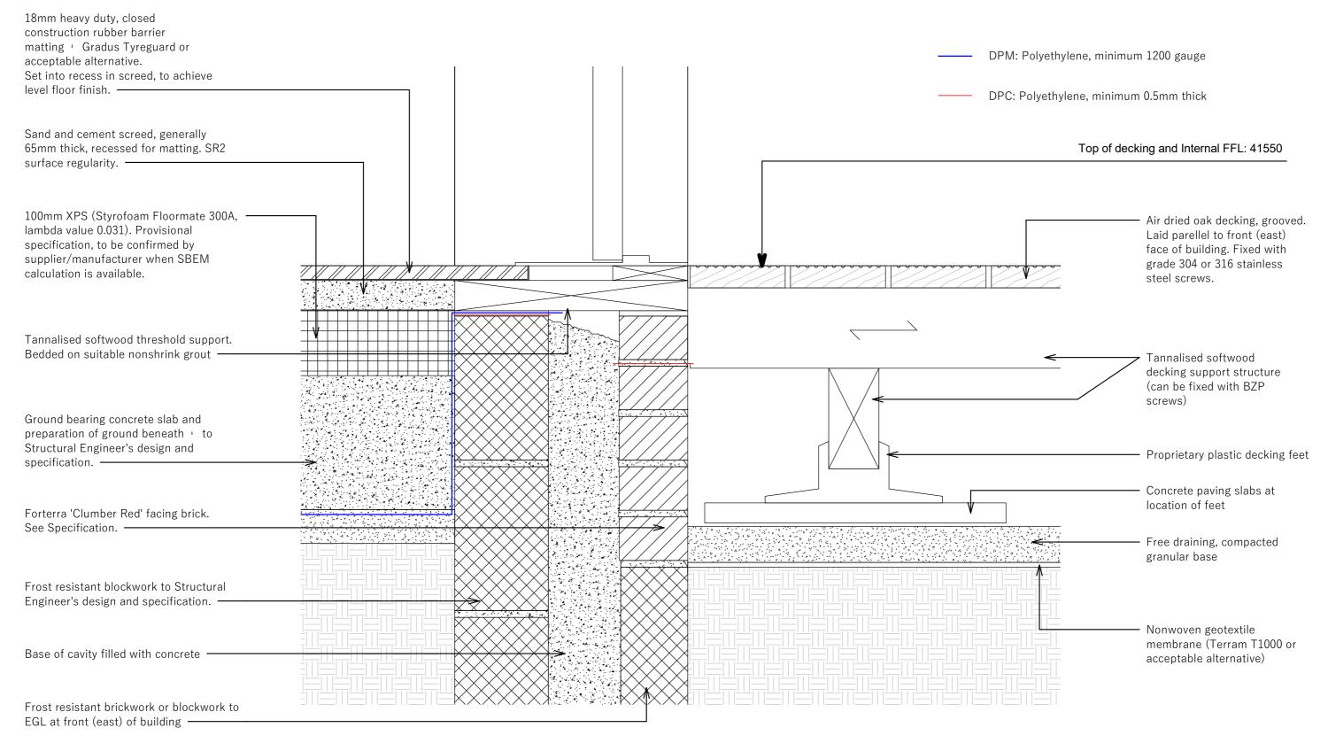
Concrete strip footing below see Structural Engineer's information
