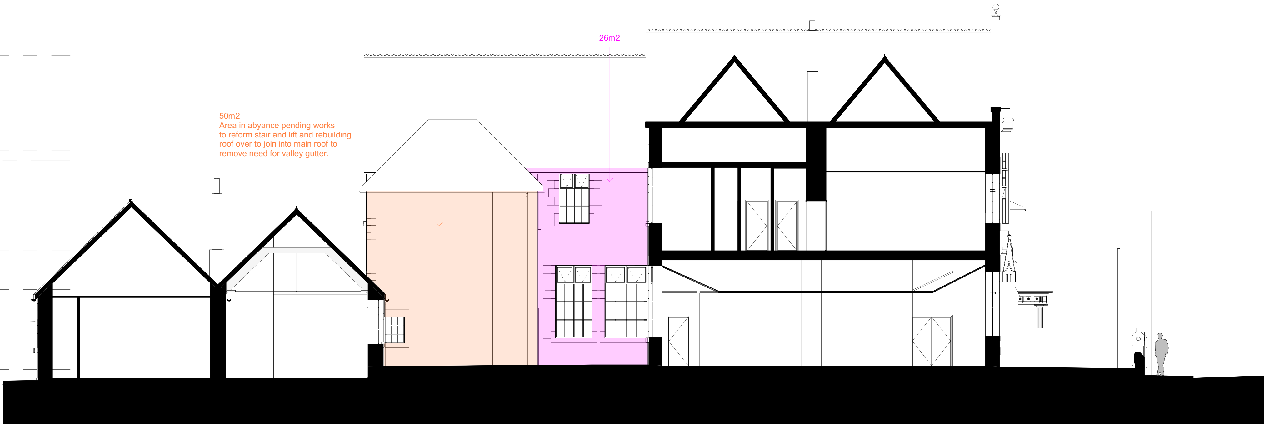
2 SECTIONAL ELEVATION - GA - EXISTING - NN - SOUTH - GRANITE FACADE REPAIR & REPOINTING 1 : 100
