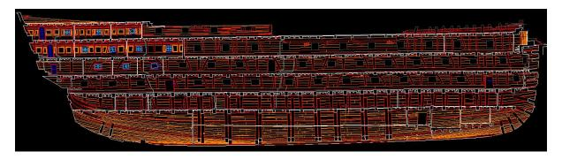
The cad profile drawings are required so that plank strakes can be accurately plotted to achieve suitable shear lines and positions of gun ports when establishing a butt plan.
