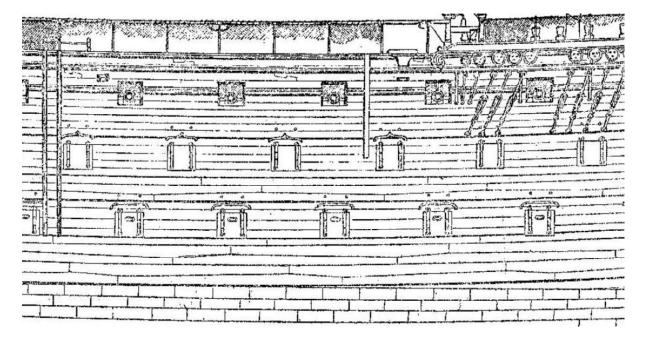
The full profile drawing of HMS Victory by G F Campbell clearly shows how the gun ports at the stern and bow cut into the wale strakes. It may be necessary to slightly increase standard plank lengths where plank stakes become interrupted by gun ports at the bow and stern to avoid short planks which are undesirable and are a weakness to the structure.
