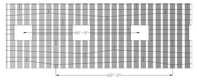
The butt plan will however vary from the perfect model a little in Victory because the gun ports do not follow the plank shear line. The deck layers and corresponding gun ports are laid with less sheer than the external hull planking strakes. This difference in sheer is also compounded by the hog of the ship.
