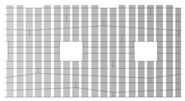
Amidships Victory's gun ports are approximately 11 feet 11/2" inch centre spacing. To achieve a suitable butt plan that avoids butts being positioned too close to gun ports it is possible that the length of plank needs to be in multiples of gun port centres. Plank length in this case would be approximately 22 feet 3". The distance between gun port centres varies a little in HMS Victory and plank lengths will vary slightly to suit.
