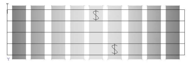
If a butt is to be positioned on the same frame it should not be closer than three plank strakes between.
