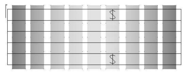
The frame spaces on Victory are approximately 16" apart which translates to a 4 feet shift of butt. This system on a vessel with greater frame spacing is sufficient but it is a little too close for Victory's shift of butt. If three frame spaces were between butts then a 5 feet 6 inch shift could be achieved.
