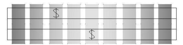
If a butt is to be positioned on the next frame it should not be closer than two plank strakes between
