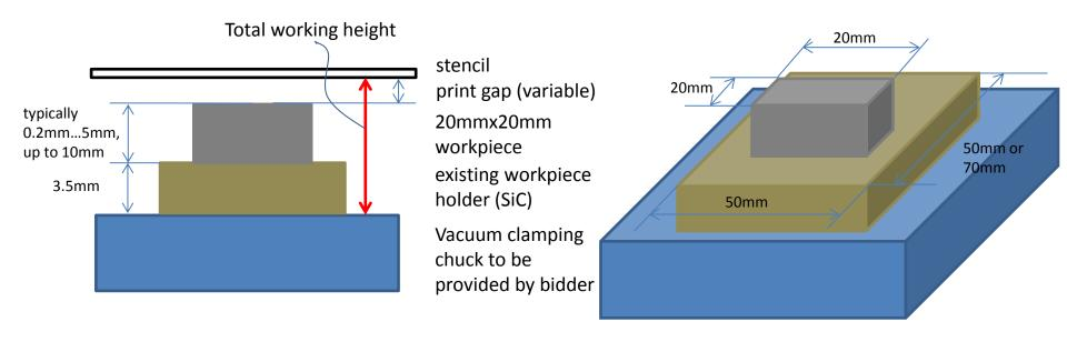
Note: The existing workpiece holder (SiC) is for a flip-chip bonder and will be transferred with workpiece to the bonder after a print. This SiC holder has got via holes which allow providing vacuum to the top surface for holding the workpiece.
