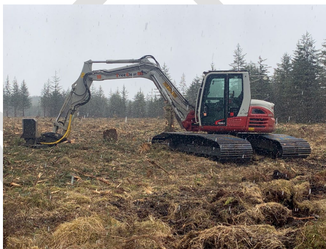
Figure 22 Low ground pressure tracked mulcher. Photo credit: TreeClear Ltd
