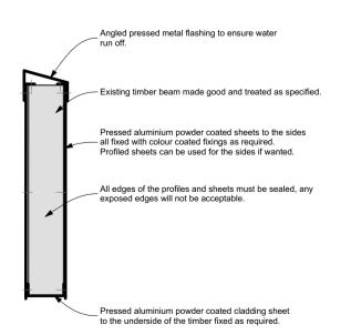
Detail through cladding of Beams
