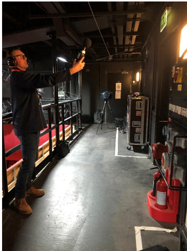
Figure D2 –Sound Insulation Testing on L01 Theatre technical gallery
