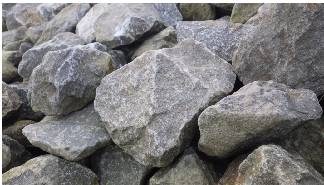
Figure 2: Kentish Ragstone used in previous embankment repairs on the tidal River Ouse.
