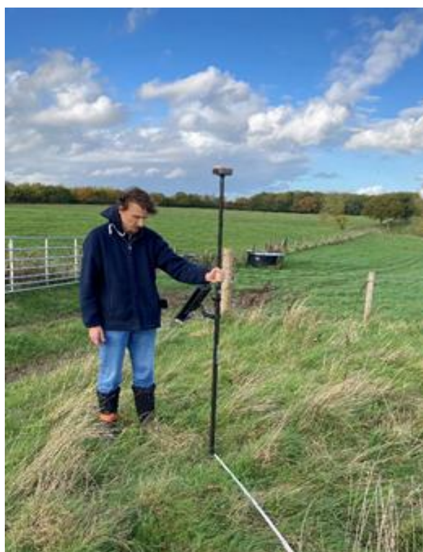
Figure 4: Locating the SW corner of location for soil classification pit using the GNSS receiver and an iPad mounted on a survey pole.
