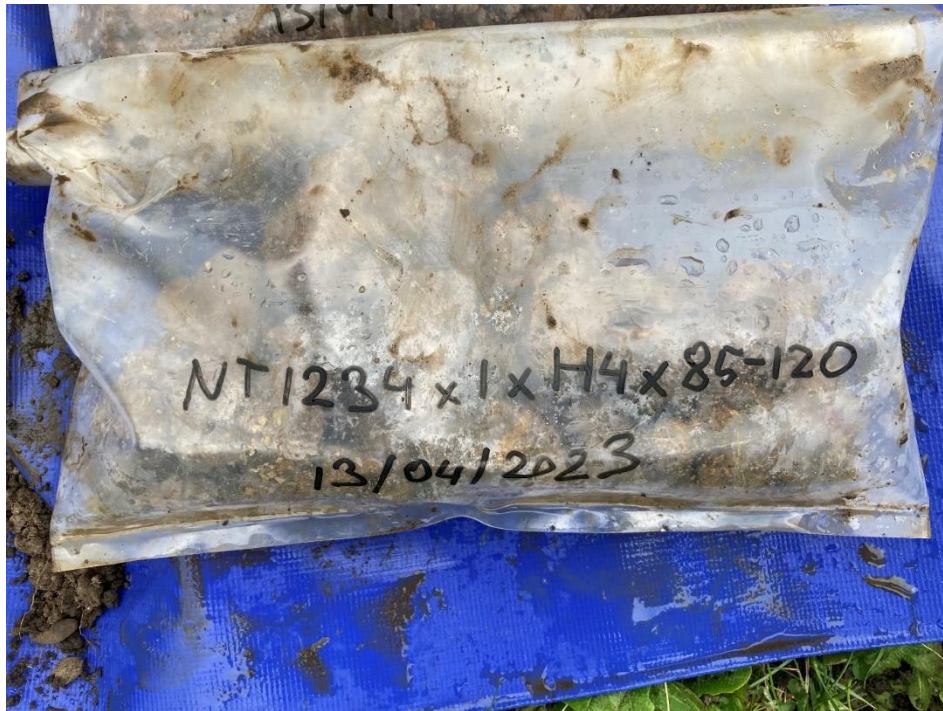
Figure 6: Sample bag labelled using a marker pen (top folded a few times, to be stapled).
