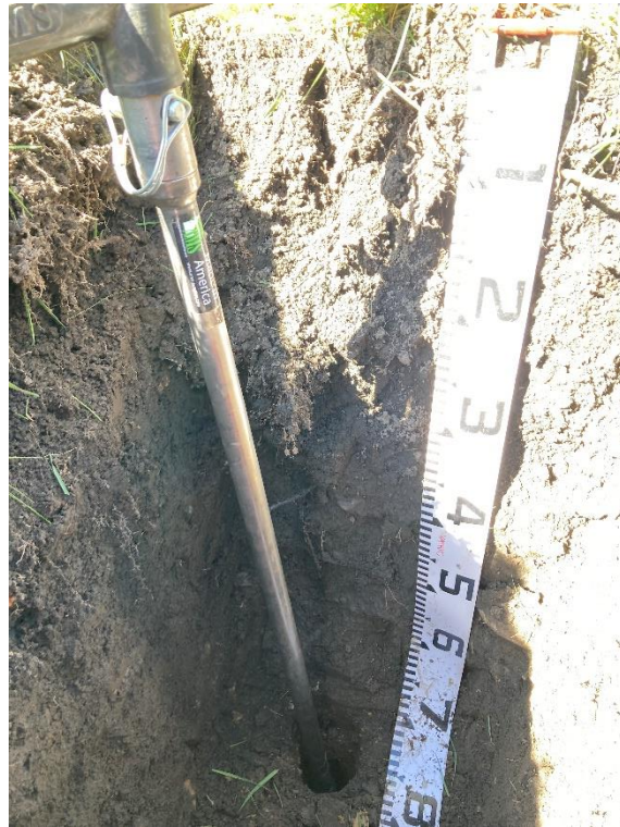
Figure 9: Coring to sample lower part of the profile.
