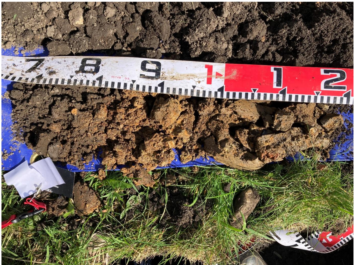
Figure 10: Soil core representing lower part of the profile (photograph recorded in the app).
