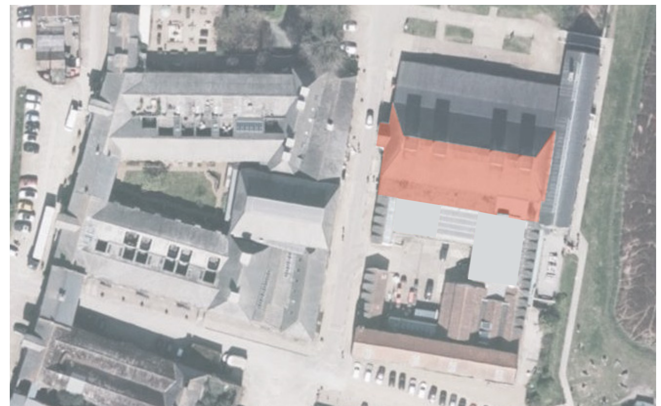
East, South, West roofs and upper flat roof require re-roofing and insulation
