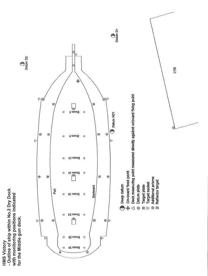
Figure 2. Outline of HMS Victory within No.2 Dry Dock with the approximate positions of the installed Deep datum's, Target sockets around the edge of the dock, additional prisms, and the on-board fixed point.
