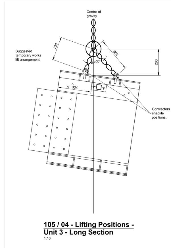
**105 / 04 - Lifting Positions - Unit 3 - Long Section**
