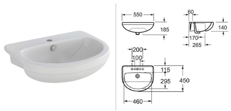
Dimensions are in millimetres except thread sizes which are BSP imperial.
