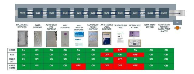
Fig.5 – Primary Kitting Cell Initial Concept.
