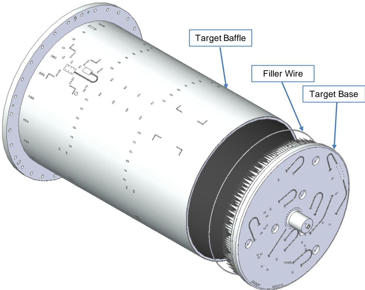
Figure 2-1 – Welded subassembly exploded view
