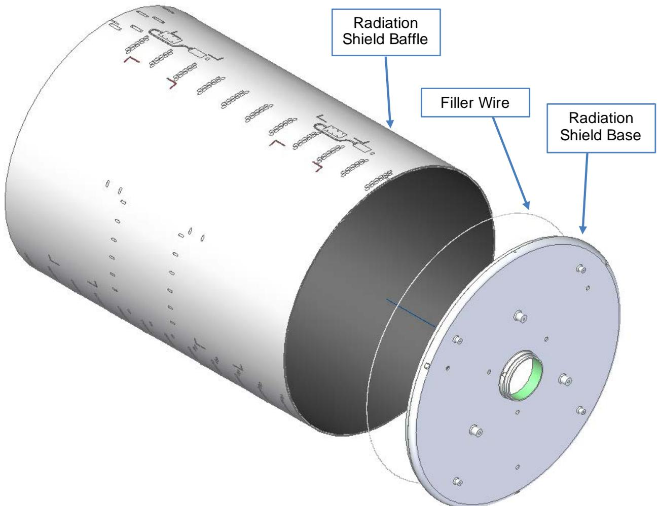
Figure 3-1 – Radiation Shield Welded Assembly (exploded view)
