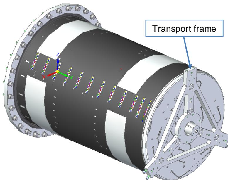
Figure 2-2 – Welded subassembly with transport frame
