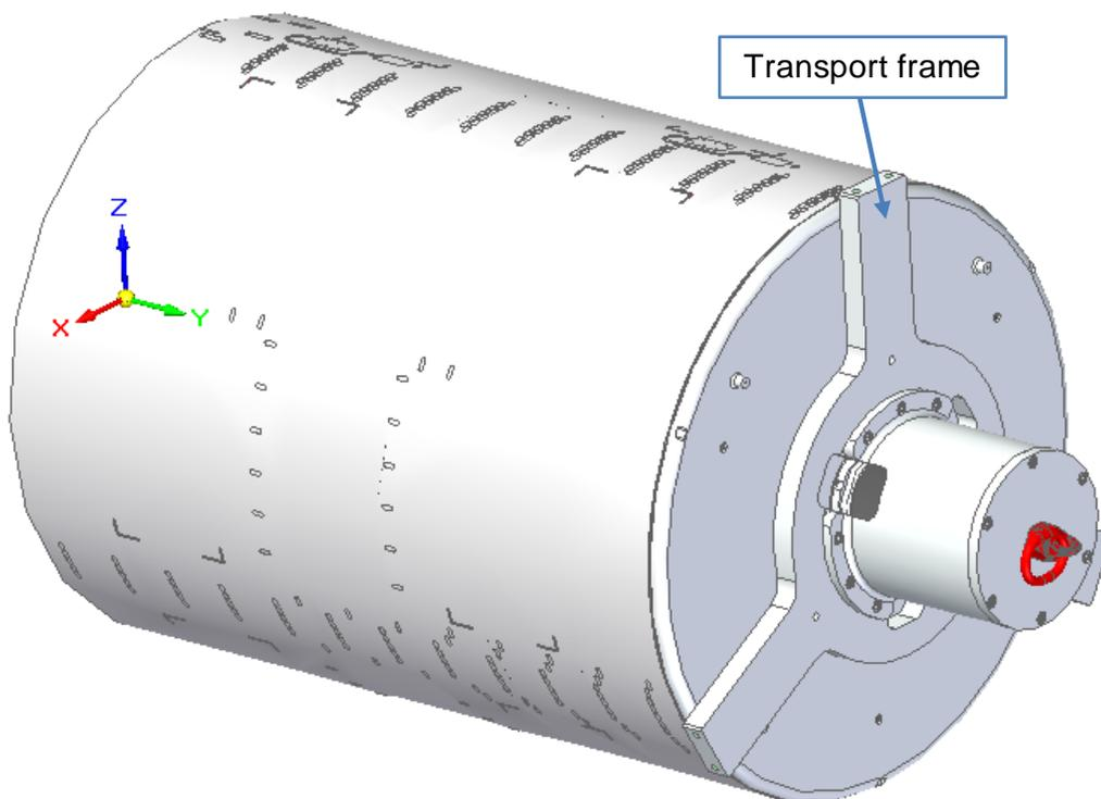
Figure 3-2 – Radiation shield with transport frame
