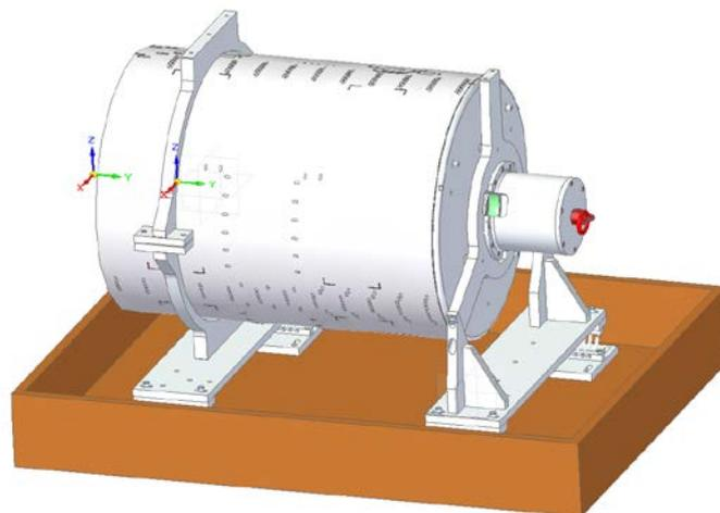
Figure 3-4 – Radiation shield transport crate (lid not shown)
