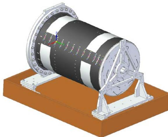
Figure 2-4 – Welded subassembly transport crate (lid not shown)
