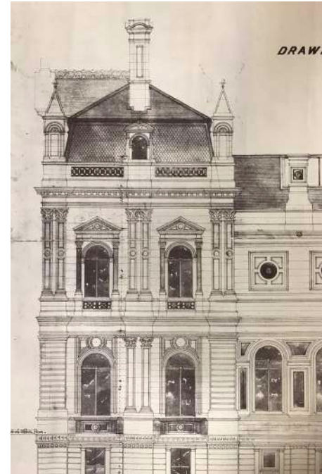
Fig.12 Deductive analysis of existing facade details, based on original drawing of the South East Elevation.
