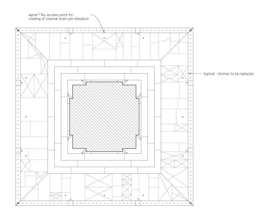
Limestone paving repairs Scale 1:50
