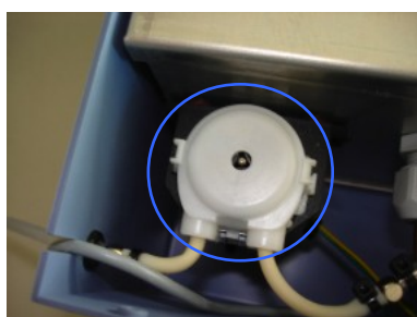
Fig. 26 - Pump head (here as built into the housing of an EBC10/11).
