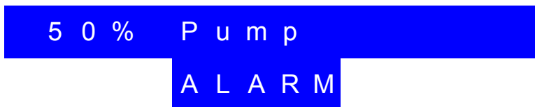
Fig. 25 - Display message for the pump alarm. The words "Pump" and "ALARM" light up rotationally.
