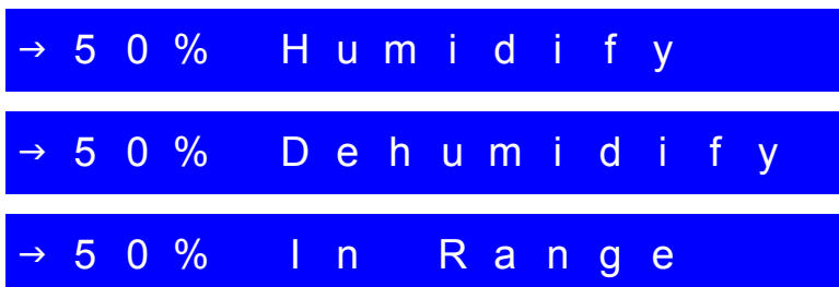
Fig. 9 - Possible display messages during normal operation (Slave sets).
