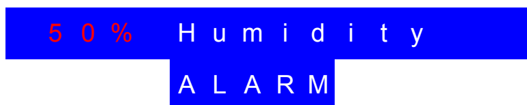
Fig. 24 - Display message for the humidity alarm. The digits highlighted in red blink. The words "Humidity" and "ALARM" light up rotationally.
