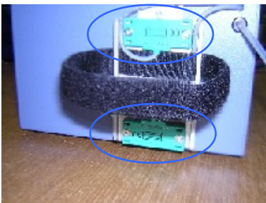
Fig. 3 - Water level sensors for the high and for the low level alarm. In the sample image, the brackets, that hold the sensors and the hook-and-loop-fastener for securing the bottle, are mounted to the left side of an EBC10 or -11. They can also be mounted to the front of any EBC10 or -11, whereas on EBC12 they are always positioned on the front plate; if you need to have them mounted to the side of an EBC12 additional parts need to be ordered for that purpose.
