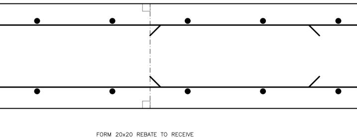
FORM 20x20 REBATE TO RECEIVE POLYSULPHIDE SEALANT (SIKA POLYSUPHIDE GG OR EQUIVALENT)
