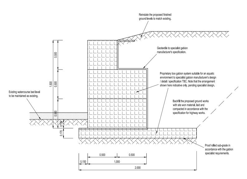
Typical Detail Through Proposed Box Gabions To Be Installed As The Re-aligned Watercourse Sides - 1:20
