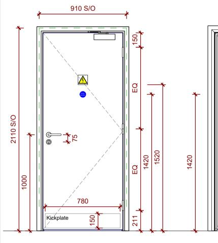
Forza Doors Ltd FD60s Flush timber doorset, paint grade finish complete with Forza pre assembled FD60 Hardwood frames.
