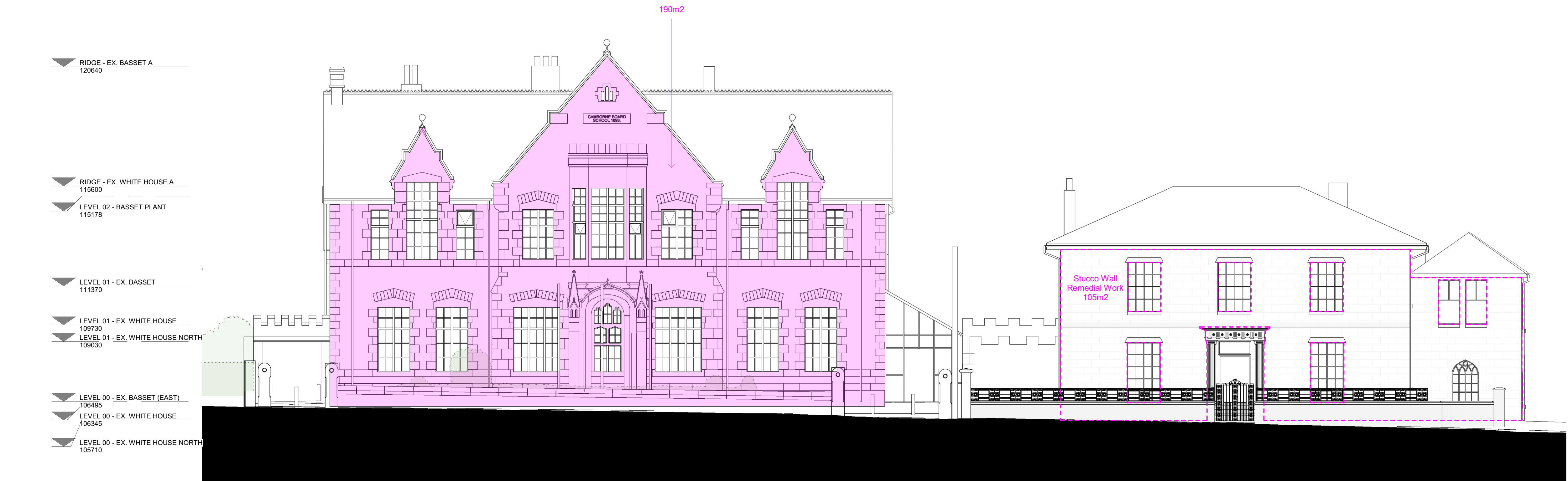
1 ELEVATIONS - GA - EXISTING - EAST - GRANITE FACADE REPAIR & REPOINTING 1 : 100
