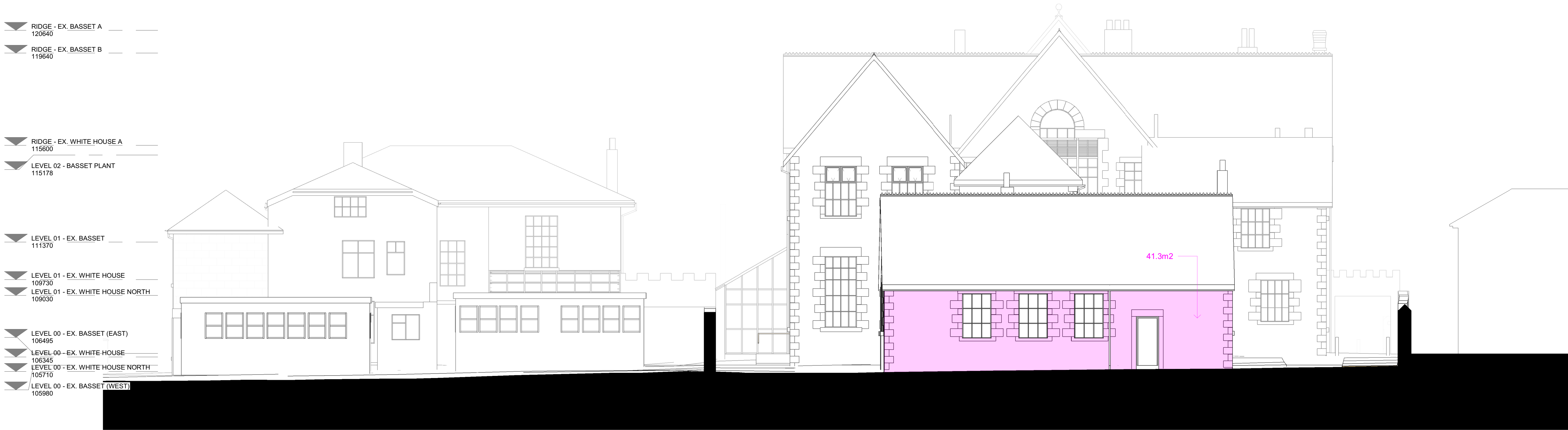
2 ELEVATIONS - GA - EXISTING - WEST - GRANITE FACADE REPAIR & REPOINTING 1 : 100
