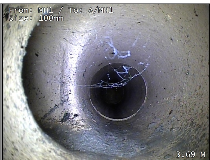
Junction at 9 o'clock, diameter 100mm
