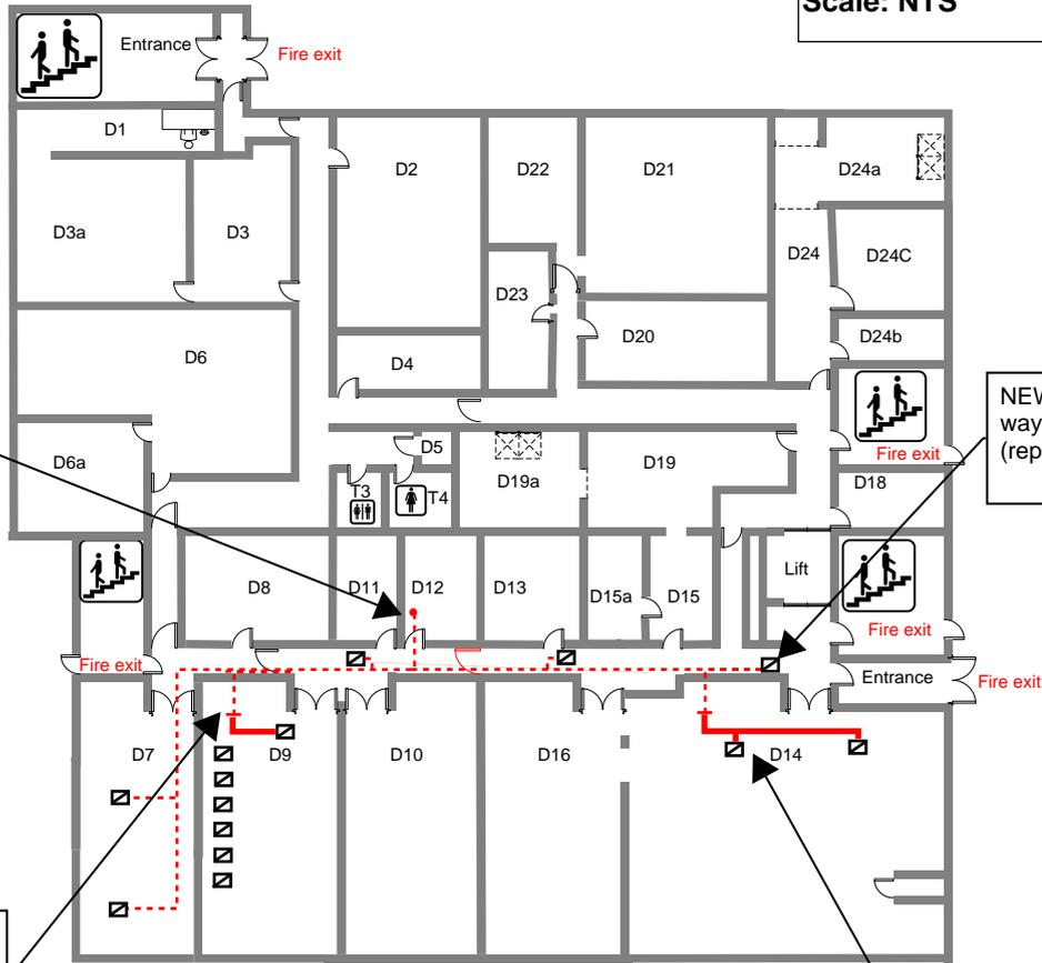
Existing supply ductwork drop from first floor. Estimated Duct Size 750mm x 400mmH
