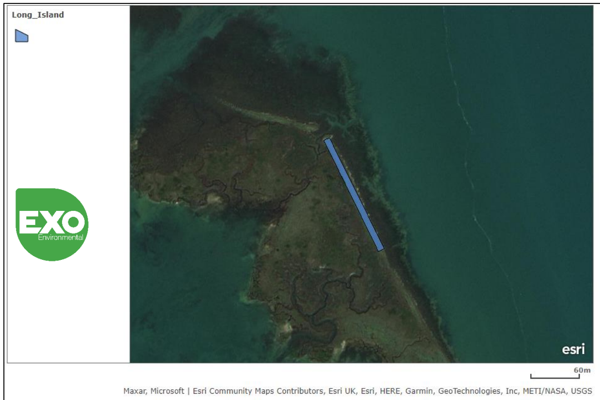
Figure 14. Long Island shingle area, which will be supplemented by 2772 tonnes to become a ridge of elevation 1m. (Esri Imagery).
