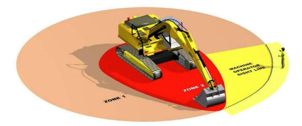
Arrangements should be that a person is not allowed to encroach inside the RED zone area until the machine has been hydraulically isolated. Everyone is expected to follow these arrangements, or alternatives with similar controls. The Construction Plant Association (www.cpa.uk.net) has published a guidance document entitled 'Reducing Unintended Movement of Plant - and managing exposure to consequential risks'
