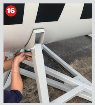
Position the stabiliser arms against the body of the model and tighten the 2 grub screws on the underside of each arm.
