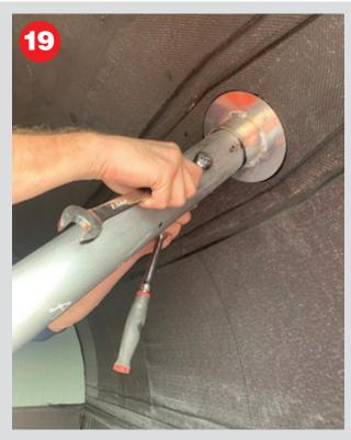
Once fitted, 2 x19mm securing bolts/nuts per fin can be fitted inside the model.
