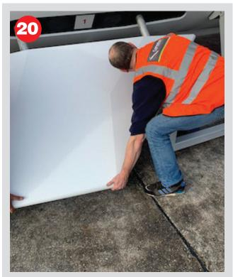
Repeat the procedure for fins 1 and 2 taking care to not allow them to scrape the ground during initial insertion.
