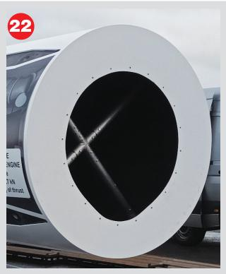
Take note that the shape of the cone is not circular and that the smaller radius should be at the 6 o clock position.
