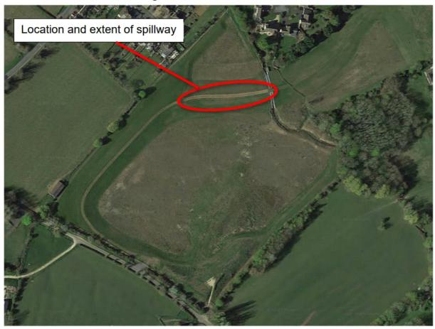
Surveying the entire length of the embankment (see image below) and ensuring the level is at 83.70 mAOD throughout (except for the spillway), topping up the embankment crest where required. Installation of overlapping gauge boards on the upstream face of the embankment on the left side of the spillway.
