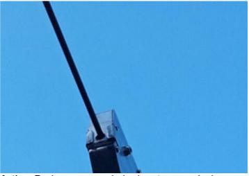
**Finding:** The nylon inserts are worn or missing at the point he cable enters the traveller **Action:** Replace worn or missing inserts as required the cable enters the traveller
