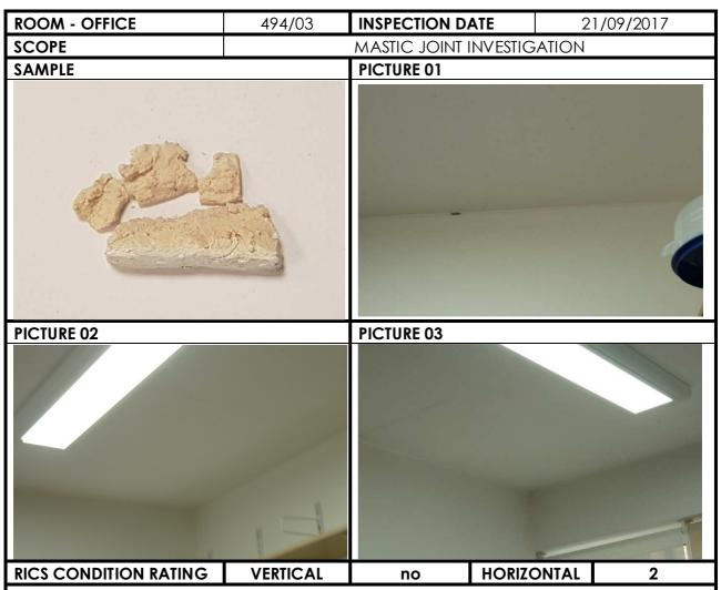
SAMPLE - Mastic joint not dry or cracked; flexibility and plasticity of sealant maintained. The movement joint width has been reduced (from expected 16mm), white foam filler (Compriband?) not found.
