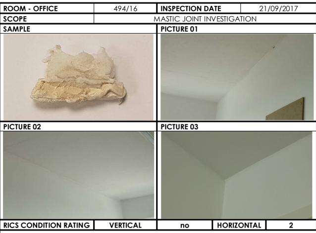
SAMPLE - Mastic joint not dry or cracked; flexibility and plasticity of sealant maintained. The movement joint width is 16mm, white foam filler (Compriband) was found, and in good condition.
