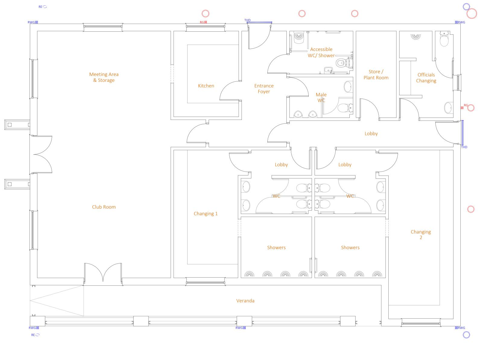
Existing Ground Floor Arrangement Scale: - 1:50
