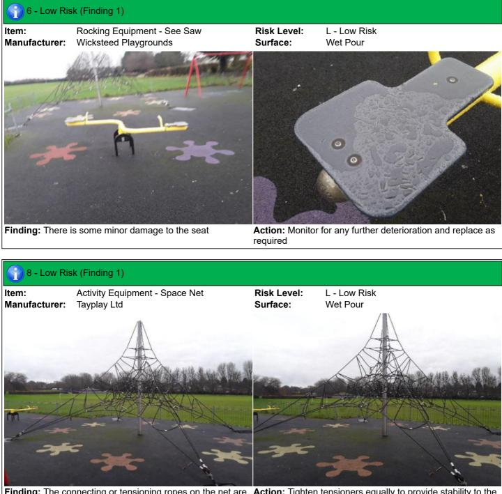
**Finding:** The connecting or tensioning ropes on the net are not tensioned correctly Action: Tighten tensioners equally to provide stability to the net structure
