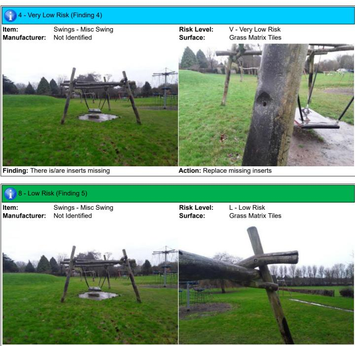
**Finding:** There are splits running through the timber that cross through or near fixing points and may cause instability in the future
