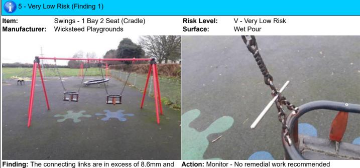
**Finding:** The connecting links are in excess of 8.6mm and less than 12mm and fail the requirements of BS EN 1176 Part 1; clause 4.2.13, Chains
