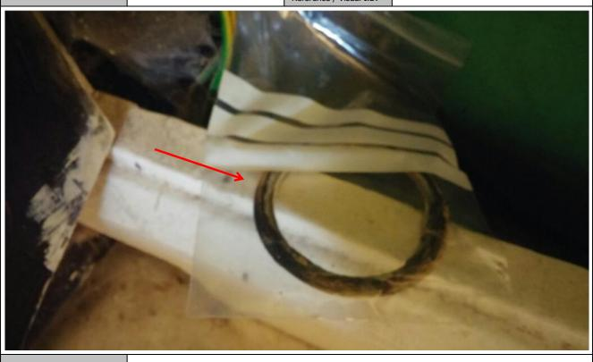
Gasket To Boiler Pipe Work Within Boxing - REMOVED AS SAMPLE
