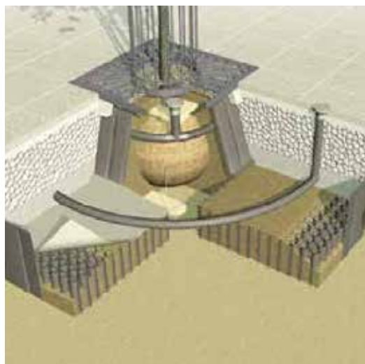
Tree pit design and the correct installation is integral to healthy street trees and the mitigation of conflict with users of streets (Greenblue,2020).
