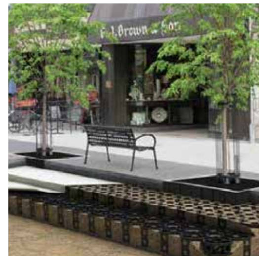
Modules help retain soil structure and prevent compaction which is essential for trees in built up environments. (Greenblue,2020).
