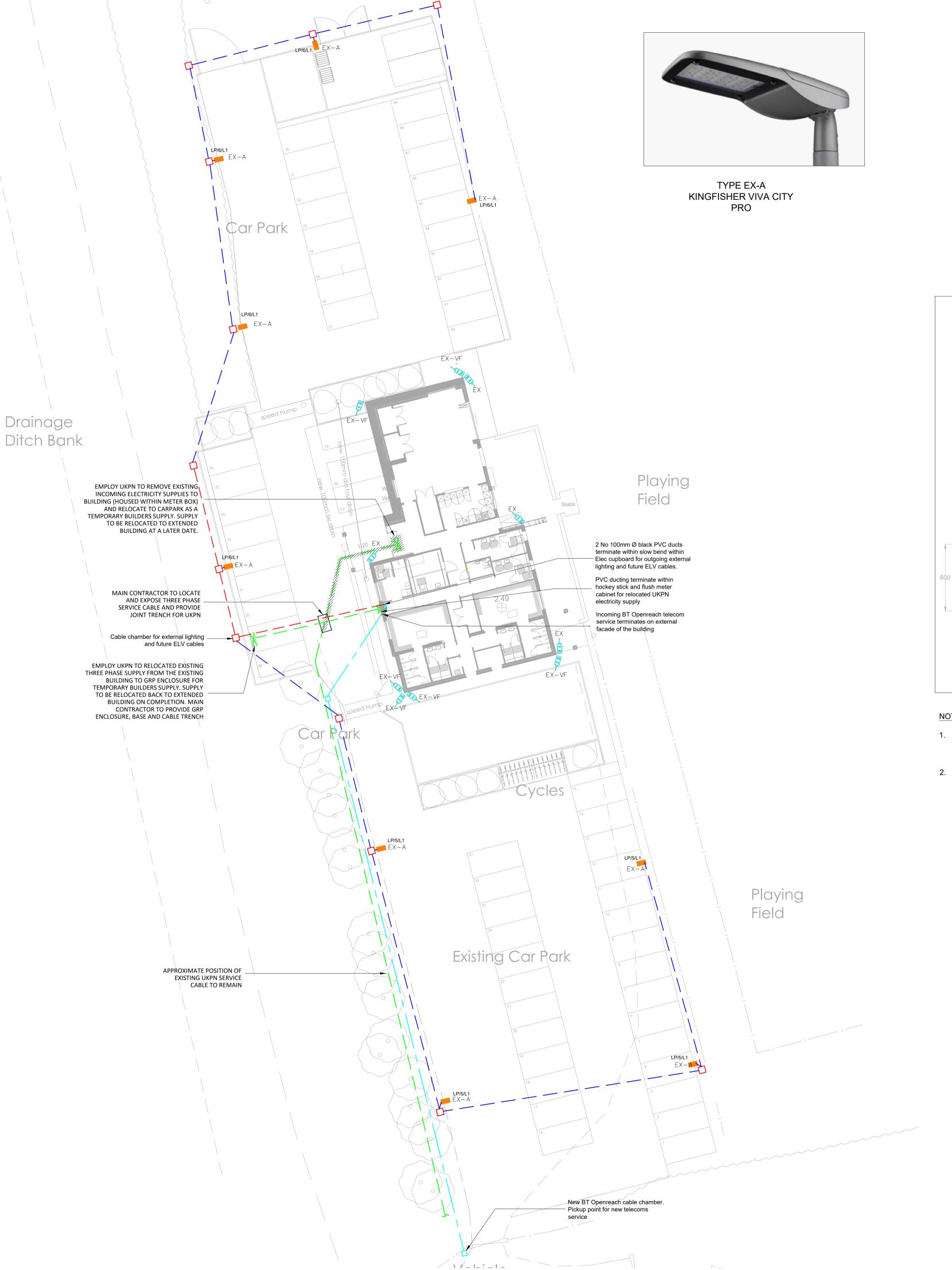
LEGEND: -2 No 100mm Ø black PVC ducts for external lighting and future use. 1 No duct to be expect clear and spare for future ELV services 1 No 100mm ø black PVC duct for external lighting mains voltage cabling. 1 No black PVC duct for Incoming UKPN electricity supply cable
