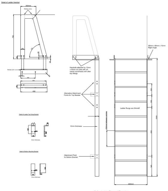
Safety Ladder Plan and Elevation
