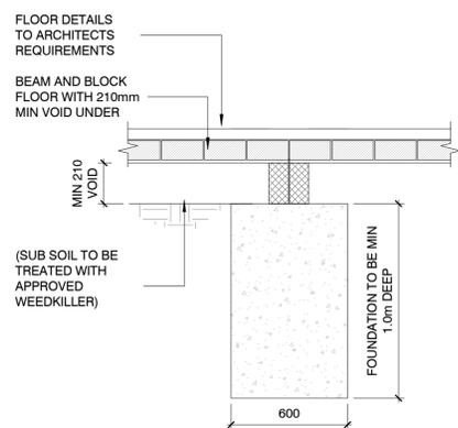
**Typical Internal Trench Fill Foundation**
