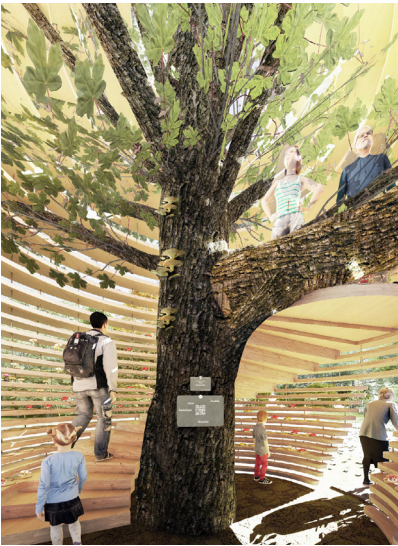
CLT corkscrew stair wraps around the tree without fixing to it
