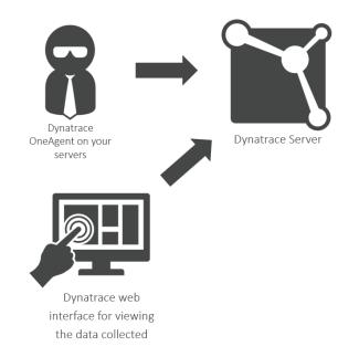
These Agents will then compress and encrypt the data captured before sending it off to the central Dynatrace Server. This server can either be hosted by Dynatrace in AWS ("SaaS" offering) or hosted somewhere nominated by you ("Managed" offering). Either way, the interface is then accessed through a web browser for monitoring or investigating issues.
