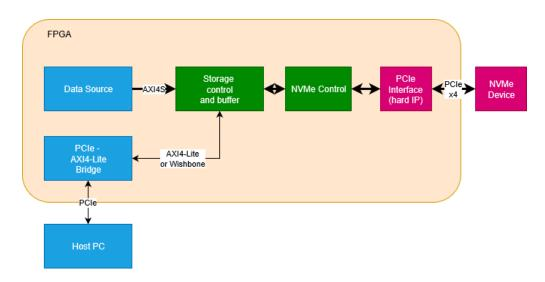
There will be a test harness either implemented in software on a host PC or on the FPGA in VHDL. The choice of this will depend on the host  $\rightarrow$  FPGA evaluation boards interface abilities of the chosen development platform.
