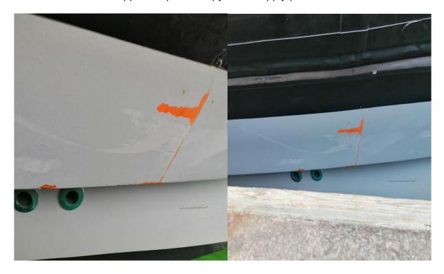
Defect 3 – Picture # 3 & 4 All Wheelhouse and Engine Room roof penetrations to be cleaned out and renewed using an approved sealant.
